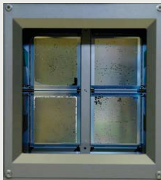
MEMS device – 105x204 micron shutters
